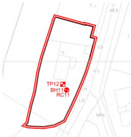
Figure 2 - Kilkenny Road Pumping Station GI locations
